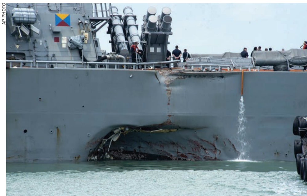
Damage to the portside is visible as the destroyer USS John S. McCain steers towards Changi naval base in Singapore following a collision with Greek merchant vessel Alnic MC
