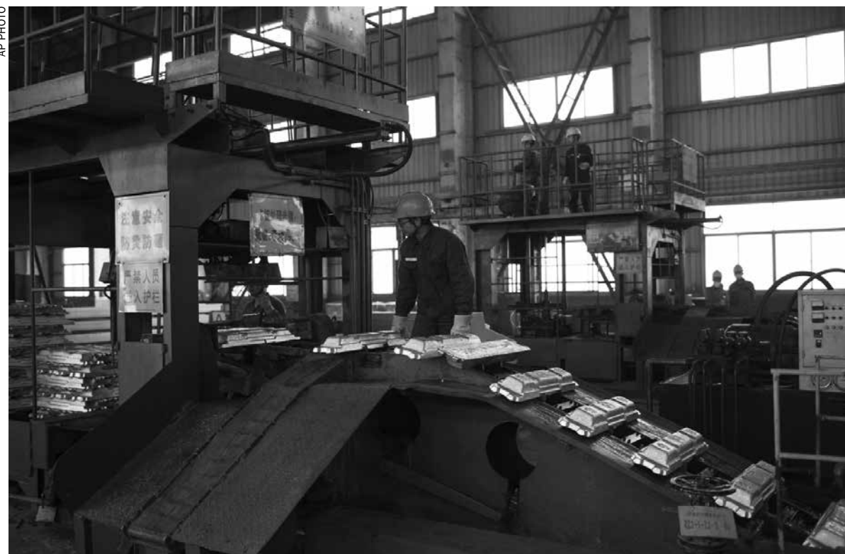
Aluminum ingots move along a conveyor belt at the China Hongqiao Group Ltd. aluminum smelting facility in Zouping
