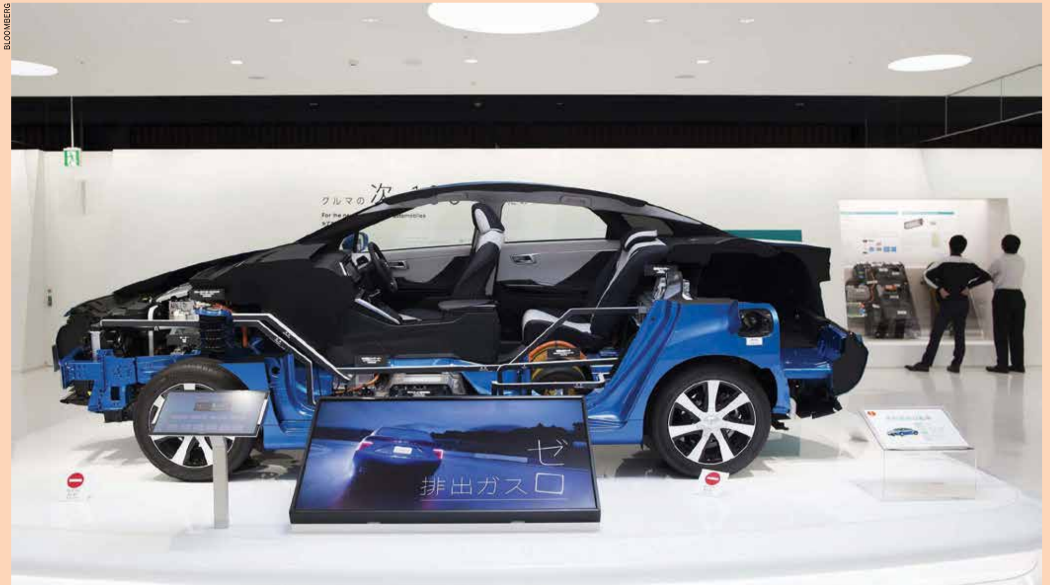
A cross section of the Toyota Motor Corp. Mirai fuel-cell vehicle is displayed in the showroom of the company's headquarters in Toyota City
