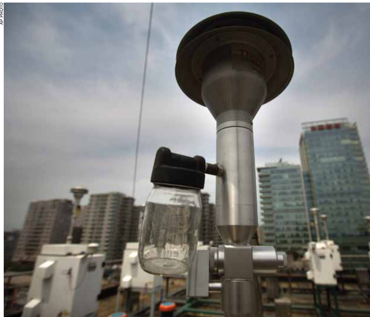
An air intake device collects air samples for monitoring pollution at the Beijing Municipal Environmental Protection Monitoring Center
