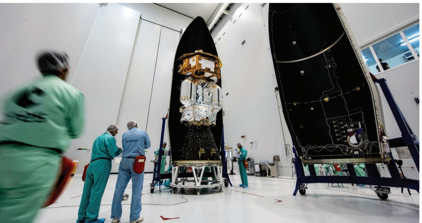
This Nov. 16 photo provided by European Space Agency ESA shows the LISA Pathfinder being encapsulated within the half-shells of the Vega rocket fairing on at the Centre Spatial Guyanais in Kourou, French Guiana
