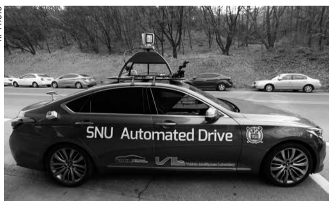
The driverless car called Snuber with a fixture on its roof with devices that scan road conditions is shown at Seoul National University's campus
