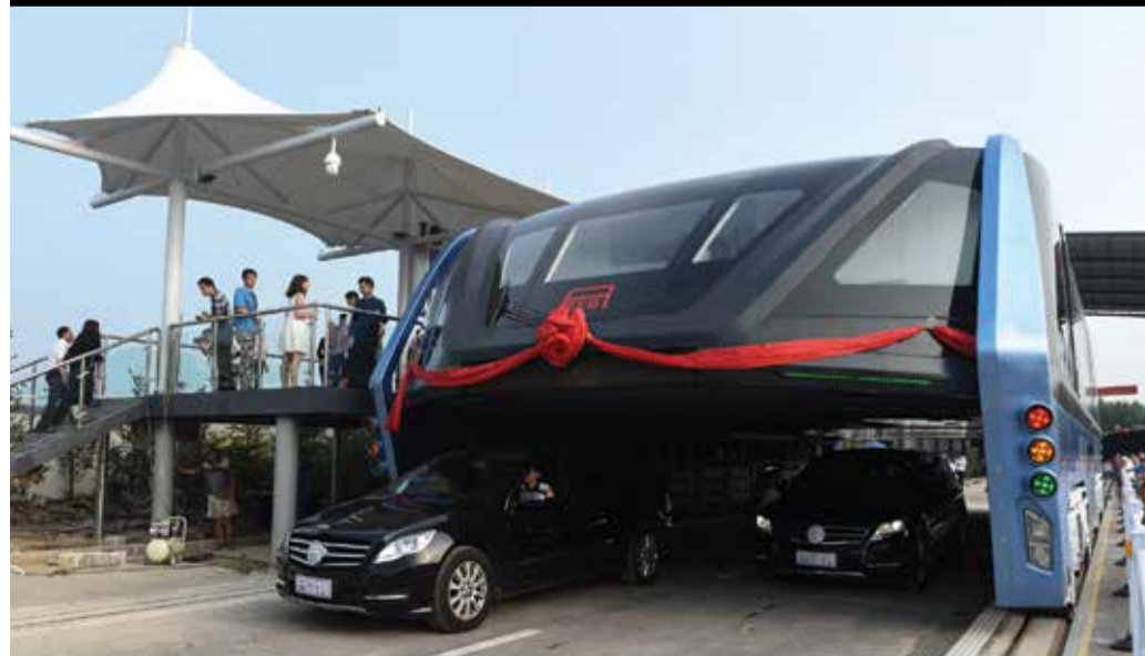
The transit elevated bus TEB-1 pictured this week during a road test in Qinhuangdao, north China's Hebei Province. The 22-meter-long, 7.8-meter-wide and 4.8-meter-high TEB-1 can carry up to 300 passengers. The passenger compartment of this futuristic public bus rises far above other vehicles on the road, allowing cars to pass underneath.
