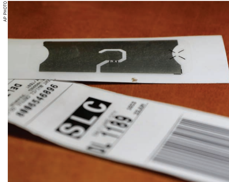
The inside of a sample RFID-enabled Delta Air Lines baggage tag
