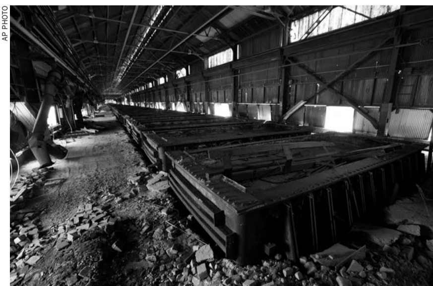
The pot line that housed the reduction cells for the former Ormet plant
