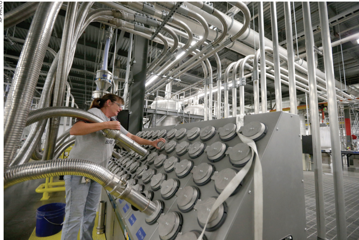
A worker moves a tube to sort recycled plastic bottle chips being processed at the Repreve Bottle Processing Center
