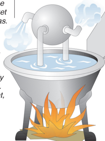
Hero's aeolipile an early steam engine
