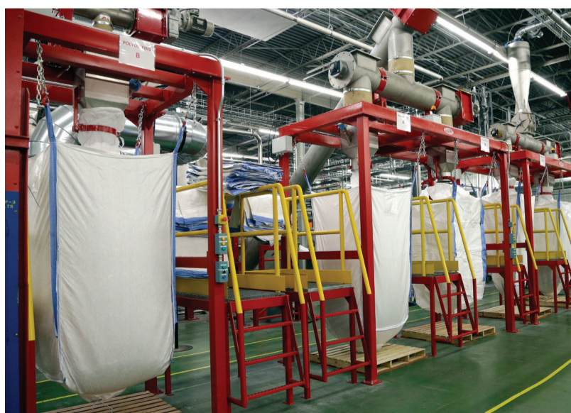
Recycled plastic chips are packed into bags for delivery
