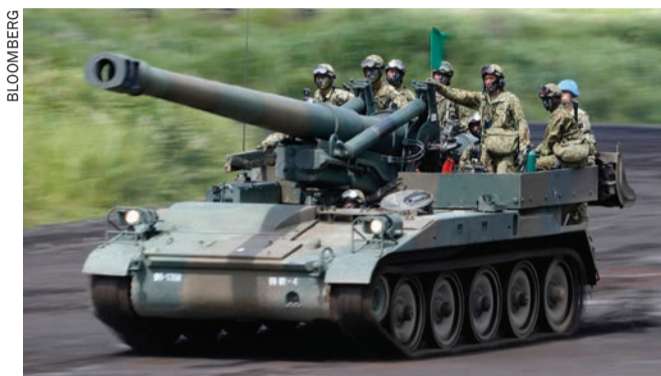
Members of the Japan Ground Self-Defense Force (JGSDF) ride a 203mm self-propelled howitzer-equipped vehicle
