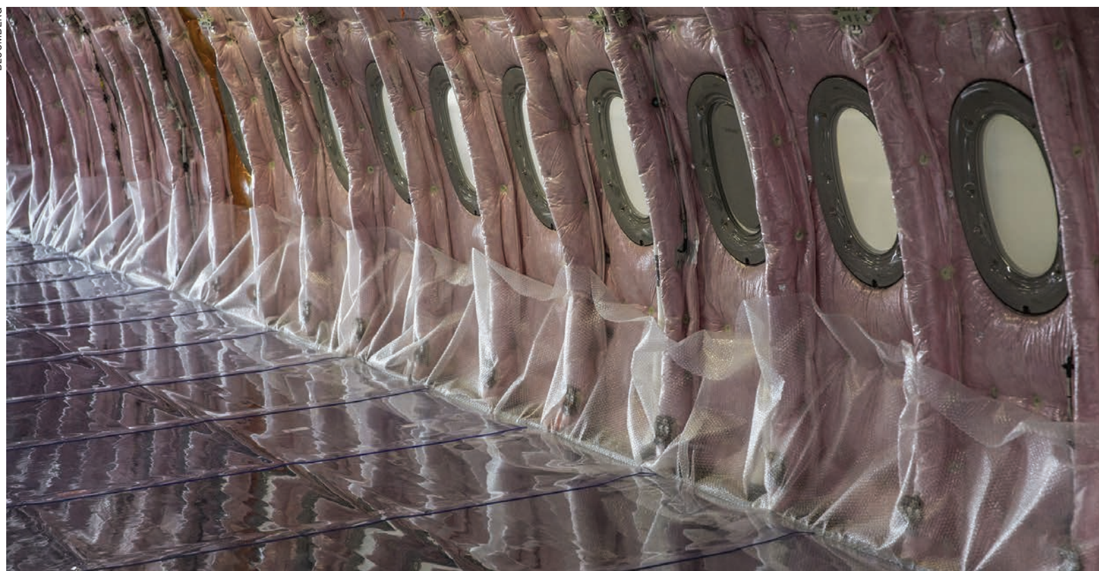
Protective bubble wrap sits in the fuselage interior of an Airbus A350 XWB passenger aircraft on the final assembly line at a factory in Toulouse
