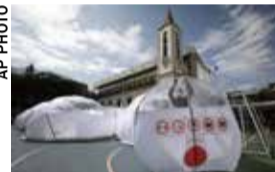
Colombia A shortage of hospital beds during the coronavirus pandemic has led architects in Colombia to design portable, inflatable chambers for coronavirus patients that can be placed in gyms or parking lots. The domes — each 5 meters wide — can house two patients and are connected by inflatable hallways. Tubes help circulate air, which can cycle through 16 times an hour, according to the architects.
