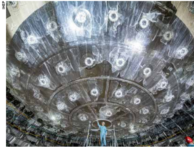
Acrylic sphere of JUNO detector (Image by IHEP)
